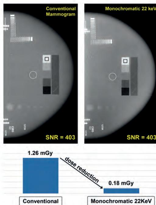
Figure 4. A 4.5cm thick breast phantom imaged with a conventional mammography unit (left) and with 22keV monochromatic X-rays from the prototype (right). The SNR for the 100% glandular step wedge is calculated for the 5mm x 5mm square outlined in black.
