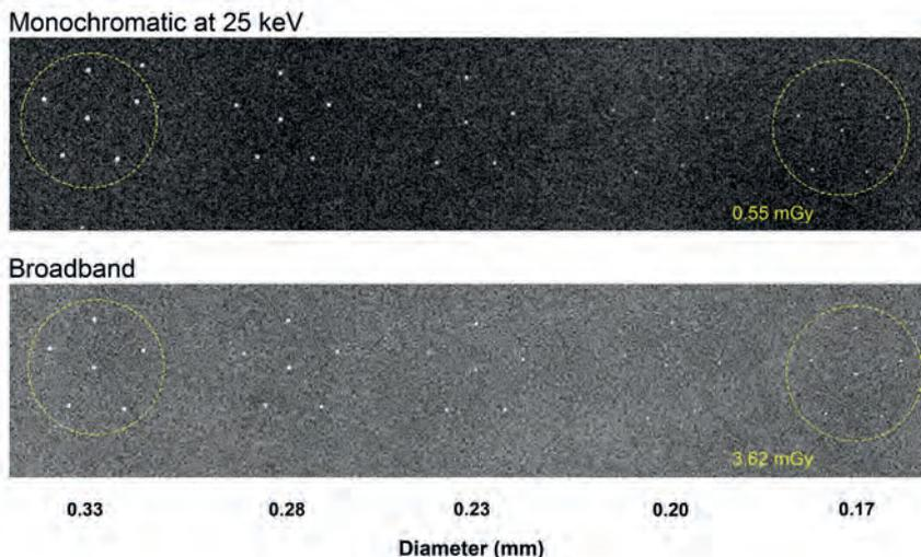
**Figure 5.** Images of simulated microcalcifications with diameters of 330, 280, 230, 200 and 170 microns in a 4/1 cm thick phantom for both instruments. The SNR values are equal but the dose of the monochromatic image is 6.6 time lower. The microcalcifications are 6 cm above the image plane.
