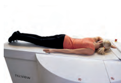
Figure 1. The nu:view Mamma-CT system was developed and is produced by the German company AB-CT - Advanced Breast CT. The design of the new scanner allows compression-free imaging of one breast at a time. To do this, the breast CT system uses a rotating gantry on which the X-ray tube and photon-counting detector are mounted. During the image acquisition process, the gantry rotates around the breast in a downwards-oriented spiral trajectory. In the course of a single scan up to 12,000 projection images are acquired. A full spiral scan takes as little as 7 - 12 seconds. The radiation dose is similar to that of conventional mammography.
