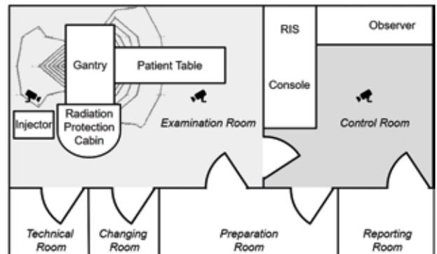
**Figure 1:** Schematic overview of the study setting in the examination room and in the control room (radiological information system, RIS). Isodose lines are sketched shaded black around the gantry. Positions of the ceiling mounted fisheye cameras are represented by the icons. Image reproduced from [10] ©.
