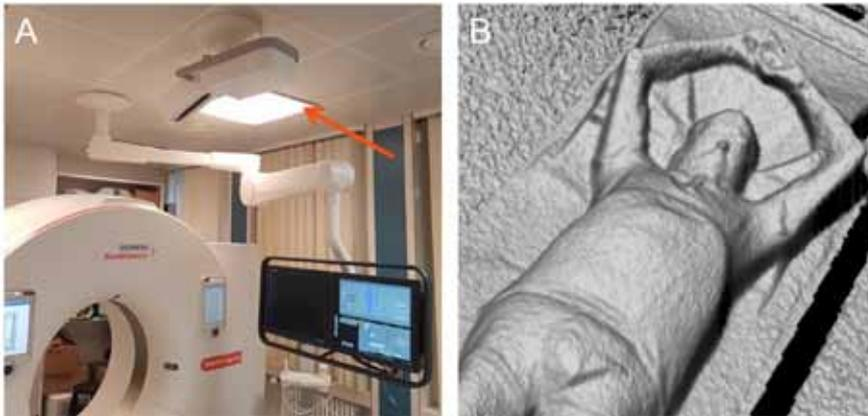
**Figure 1.** (A) The 3D camera (Red arrow) placed above the CT table; (B) 3D surface image of the patient obtained by the 3D depth camera.
