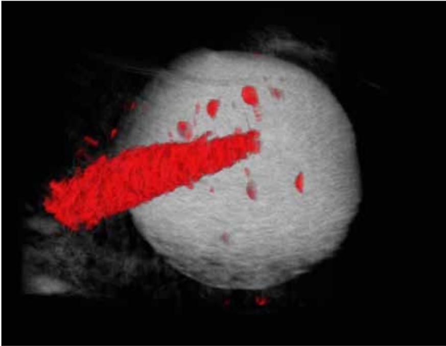
**Figure 2:** Volumetric ultrasound data of custom phantom target (gel sphere and flow channel) rendered in 3D. B-mode data shows reconstructed sphere in the background; color Doppler data reveals flow channel in the foreground.
