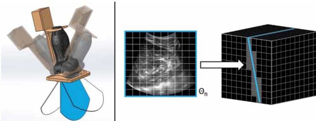
**Figure 1:** (left) Diagram: 3D volume acquisition sweep with probe fixture and orientation sensor; (right) diagram: 3D volume reconstruction method. The fixture establishes a pivot axis, and the sensor (box at top) returns orientation readings as the probe is tilted and the image plane (below) is swept through the body; each recorded 2D image plane is inserted into the 3D voxel according to its orientation reading.
