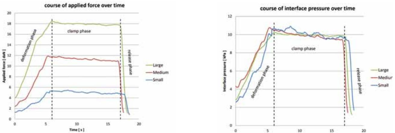
**Figure 3:** Real time recording during a typical mammographic compression with a dedicated paddle with a contact area measurement tool. The ratio with the force contact-area is calculated to the mean target pressure (10 kPa) [6]. Women with small breasts receive a lower force according the output of the mammographic machine but undergo the same pressure.
