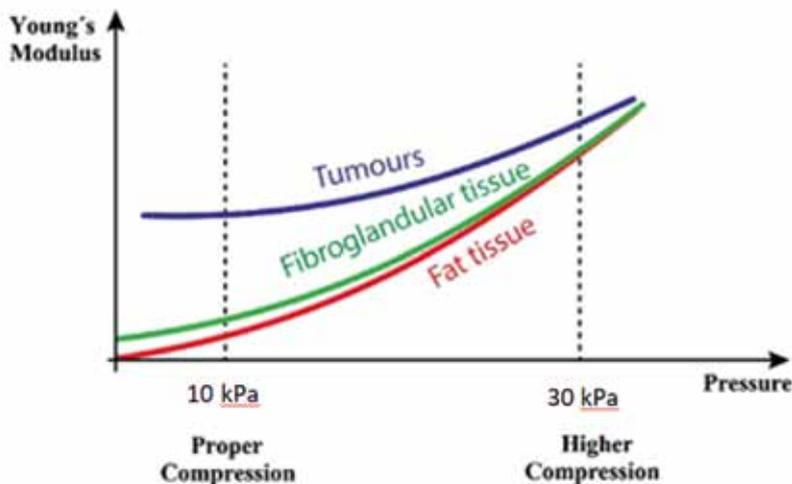
Fig 5. Converging stiffness curves at increasing compression pressure (Adapted from 13, 15).
