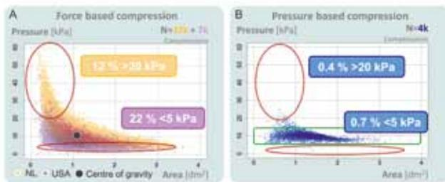
**Figure 4 :** A: under the current way of working as calculated from a database (US and Dutch data), a large variation in pressure can be noted, in which the 20 daN limitation of the motor-drive of the paddle explains the banana shape of the plot. In fact women with small breasts are in no way protected by this limitation. B: Same plot as A in a hospital population with application of a pressure based compression. Figure adapted from [10]
