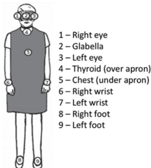
**Figure 1.** To estimate absorbed doses, nine pairs of thermoluminescent dosimeters were used
